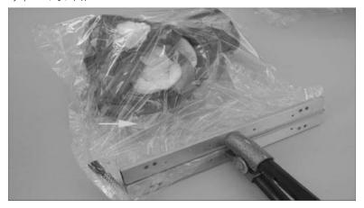
**Figure 7.**Rubber gas mask being enclosed with oxygen absorber (indicated by white arrow to left of picture). The oxygen impermeable bag is flushed with nitrogen just prior to heat sealing closed (tube to nitrogen cylinder is clear to left of heat sealer).
