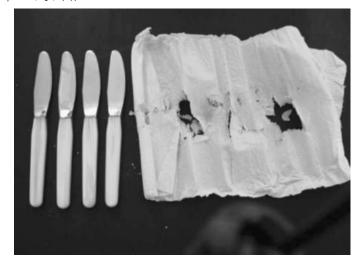
**Figure 3.**Acetic acid produced by degrading knife handles from the 1950s, has 'burned' the paper in which they have been wrapped during storage. The knife blades have also undergone corrosion on contact with acetic acid.
